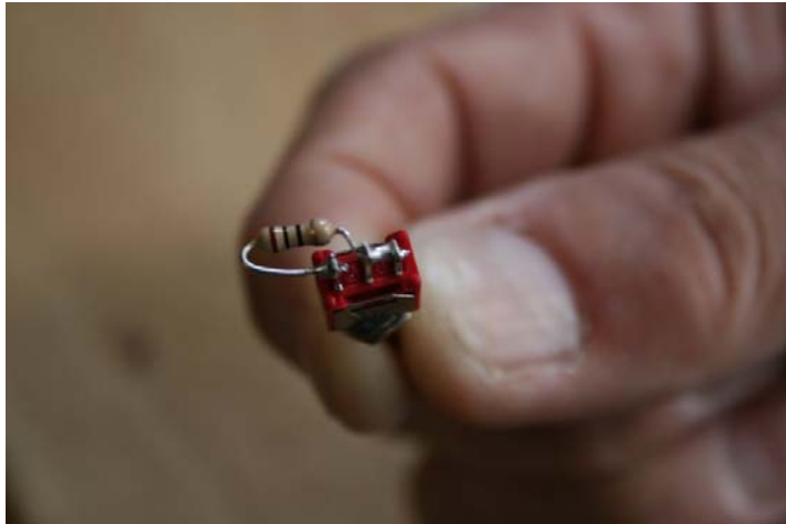
Photo 4. Close-up of connection details of the toggle switch
