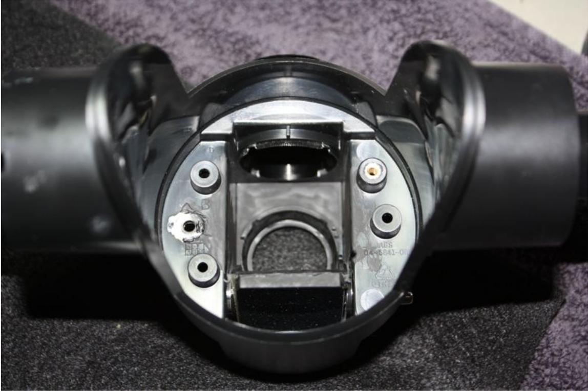
Notice the small washer glued over the hole on the left. It has been painted over a bit with flat black paint, but you can see here how it is attached.
