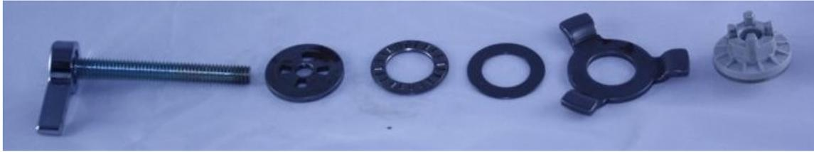
This seems to be a slightly larger problem. And to be honest, I found a much easier way to adjust this on my last disassembly. This clutch works similarly to the vertical with a few extras. The large lever turns bolt that squeezes down on a 3-pronged washer that in turn puts pressure on the horizontal drive clutch. The adjustment of this bolt, and the breaking of the internal castle nut are the critical elements.
