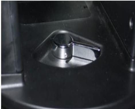
The key to getting this clutch to work right requires proper assembly and setup. First, remove the set screw that holds the chrome plastic lever onto the bolt. You can see the set screw by moving the lever to the right.
