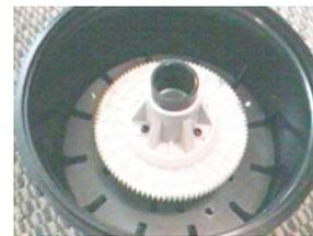
36) Apply a small amount of grease to the worm gear under the base. Apply a small amount of grease to the metal shaft, and then replace one of the nylon bushings.
