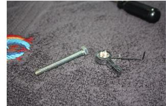
After removing the lever cap, flip over the scope and remove the bottom access cover. Remove the locking bolt and the clutch assembly will fall free leaving the white castle nut. Carefully remove the white plastic nut.
