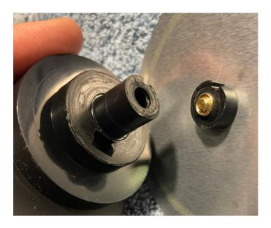
My goal on this was to place threads inside the hole in a way that would both create threads and add strength. Then to re-attach the small broken plastic ends to the axle and make it look as close to the original as possible.
