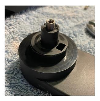
Next, I super glued the other two pieces in place against both the standoff and the plastic of the broken axle top. I was comfortable with just gluing this as the forces it experiences in operation are compressive and it should handle that well. I had to file out the insides of the two pieces to get them to fit well. I then glued them and squeezed them in place with a clamp to ensure they were well seated:
