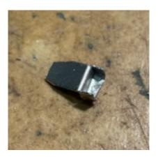
I then soldered the corners of the part to give it added strength. I angled the sides of the flat tab to allow it to penetrate into the plastic and accommodate insertion. This beautiful little part was exactly what I had in mind:
