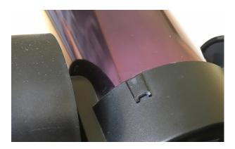
I wanted to fix this mount but also wanted it to look as original as possible. This required shaping the mount channel so that I could embed a reinforcement piece inside the raised plastic mount base instead of bolting or gluing something on top of it. After lots of thought I envisioned a part that looked like this:
