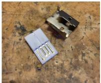
From this USB metal, I used pliers to bend it and tin-snips to cut it into a T-shape:
