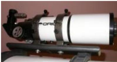
The clamshell adjustable mounting rings are available from Scopestuff and the deluxe knobs and reticle eye piece are also from Orion. The diagonal is a StellarVue enhanced 1.25" diagonal.
