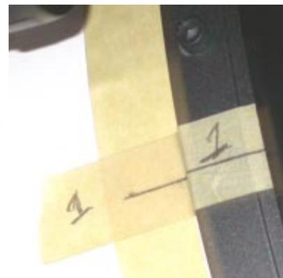
Before starting tape and mark all of the indexing marks for correct replacement of the corrector and primary cells when finished. This procedure is detailed in the Ultimate Collimation Guide (UCG).
