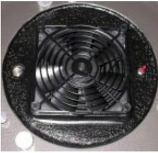
other ring with the screws, washers and locknuts. The side of the disc with the DynaMat treatment will face the outside of the primary cell. The fan has mounting holes on both sides. Depending on what side you use to mount it, the fan will either protrude further into the OTA or protrude on the outside of the
