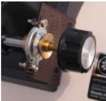
This modification is designed to solve the problem of fine focus adjustment on the SN10 stock focuser. The result is a vast improvement over the stock focuser. The focuser will feel firm yet smooth. You can still perform macro movement with the remaining original knob plus you will get 6:1 fine tuning
