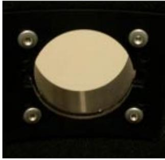
If you are mounting the stock focuser back onto the scope, only mount the base - remove the focus tube, and pinion / knob assembly. Stuff some paper towels down the focuser or mask it off with masking tape to keep the paint from drifting up the focuser tube and out of the OTA.
