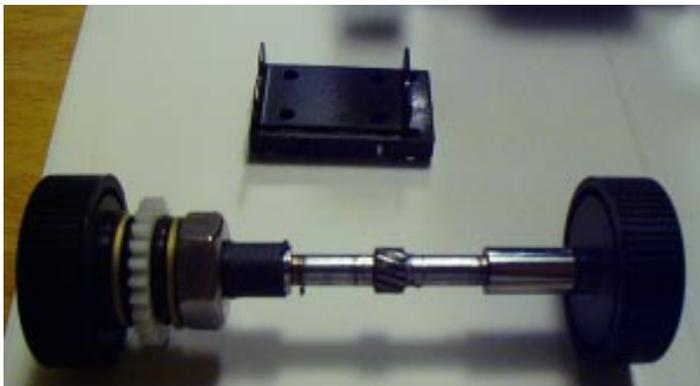
knob, clutch flange, o-ring, nylon gear, o-ring, brass washer, nut. This assembly will slide back over the pinion shaft.
