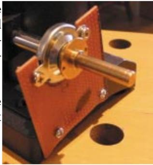
11. Mark the position of the attachment lugs on the circuit board. Drill holes for the bolts.
