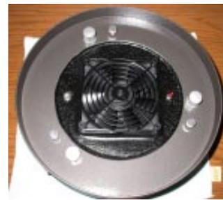
If you look closely at the three large primary mirror adjustment screws on the rear cell in the picture, you will see that there is a white nylon washer under each of them. I found that this along with a very small dab of white lithium grease or Lubriplate resulted in much easier and smoother
