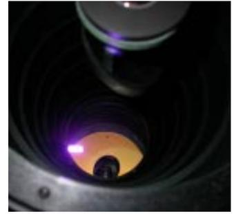
If you own a refractor, you can also reap the benefits of OTA flocking. If you remove the front objective cell and the rear focuser cell, you will notice that the OTA has several circular baffles already installed. I covered the inside of my AR6 from the first baffle to the end of the OTA at the objective end and from the last baffle to the end of the OTA at the focuser end. I used the self adhesive backed black velvet - product #88015K33 - available at:
