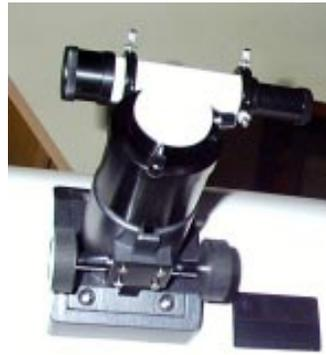
Take a piece of shrink tubing and cut it to fit over the end of the pinion shaft with the knob removed. You want it to cover only the large end portion of the shaft. Leave about a 1/16 inch gap of metal showing at the inside flange – do not cover all the way to the center smaller shaft. Leave just enough hanging over the end with threads so that it “wraps” over the shoulder of
