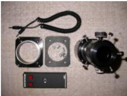
Mounting the new focuser was a piece of cake. Total time was about twenty minutes with another ten minutes to align it to be perpendicular to the tube. A task made very easy since the base includes four collimating screws to fine adjust the orientation of the focuser.
