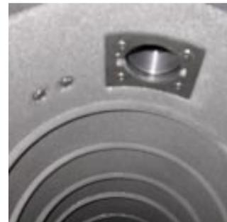
Before painting the inside of the OTA with the Ultra Flat Black paint, you want to mount all of your accessories back onto the tube. This includes the finder scope, focuser and anything else which has bolts passing through to the inside of the OTA.
