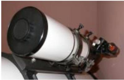
I chose the Orion ST80 (80mm f/5) wide field scope to use as my finder and guide scope on my SN10. I still have a red dot reflex finder mounted on the ST80 for quick positioning of the scope. I use a 12mm double crosshair illuminated eye piece which is what is usually mounted in the ST80. It's a very nice little scope with wide field views and works well. Eventually, it will probably be fitted with Meade's LPI AutoStar Suite to be used as an AutoGuider.
