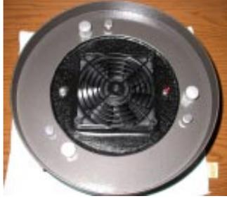
I used a 24 volt DC low profile reversible box fan. The 24 volt fan allows me to choose 6v, 9v or 12v power taps from my power supply to vary the speed of the fan as needed. Select the thinnest fan you can find so that it will not protrude beyond the rear of the primary cell when you are finished. This will allow you to still be able to stand the OTA on the primary end should you need to store it.
