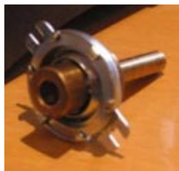
*Note: The reduction drive (pictured) is designed to allow fine tuning of air*
