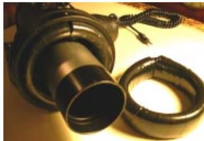
Make sure it clears the rack and focus tube. The picture shows the ring mounted inside the focus cell of my Orion 120mm f/8.3 refractor - but also works with the AR series of scopes.
