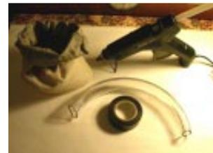
Carefully remove the focus cell from the OTA. Cut a piece of the vinyl tubing just long enough so that you can wrap it around the inside of the OTA. Cut an additional 1/16" off of one end of the tubing.
