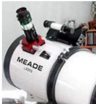
One user has used the MoonLite focuser on his SN6 and reports that the MoonLite does not fit the SN6 focuser hole from stock. The focuser opening had to be made wider by approximately 1mm and the mounting screws do not match the stock mounting holes.
