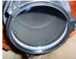
I also replaced the three bolts on the inside of the OTA which actually are in the light path, with flush mounting t-nuts as I described in the SN10 process. These are easy to get to by removing the entire front lens assembly from the front of the OTA.
