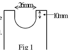
10. Cut out the semicircular shape with a coping saw. The board should fit snugly around the outer case of the drive, allowing enough material to attach the screws to.
