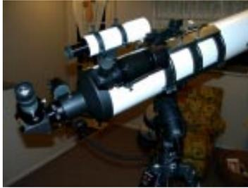
Another finder that I have mounted on all of my scopes is the red dot reflex finder. These add almost no weight, are low profile and make pointing your scope just that - point and look. They consist of wide field of view lens which has a red dot projected on it from a LED. The brightness is adjustable to suit your viewing conditions. If you can see an object, you simply move the scope till the red dot is on the object - it doesn't get any easier than that.
