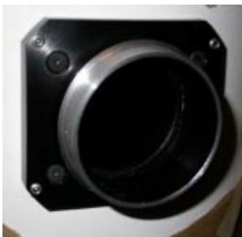
After removing the front corrector cell as described in previous sections of this guide, you simply remove the four bolts holding the stock focuser in place, and replace it with the base and gasket using the black flush mount beveled screws provided by JMI. I placed the gasket provided by JMI between the base and the
