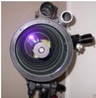
As you can see the result is a very dark OTA - even when a close-up flash is used. This increased darkness will result in higher contrast views when trying to pull out that last bit of detail in those faint fuzzies. It especially helps in light
