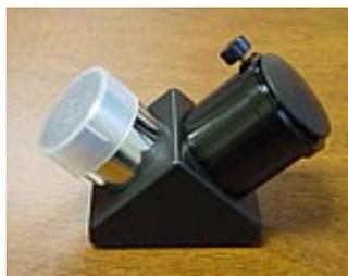
Another exceptional value in refractor diagonals is the 2" model available from Williams Optics. It has a precision 1/10 lambda surface with 10mm-thick mirror, 2"-1.25" adapter with copper clamping ring, reflectivity rate 97.0 percent, Inside diameter (48mm) includes the capability to connect a variety of filters, weight : 470 g.
