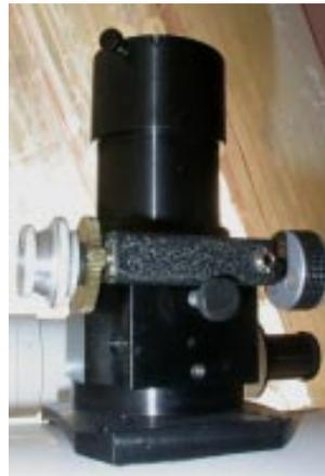
Once the base is mounted, add the focuser, insert your laser or crosshair sight tube and use the collimating screws in the base in conjunction with tightening the four main mounting screws to adjust the tilt of the focuser so that your crosshair or target strikes your alignment target on the opposite side of the OTA as described in the previously released *Ultimate Collimation Guide*.
