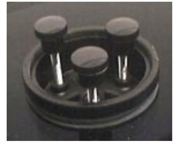
If you can't find the screws in the correct size you can buy 1/2" female threaded knob heads and a threaded 3" 8-32 rod and use a Dremel to cut them down to size. I used the Dremel to grind the end of the screw smooth so you get a nice even contact with the secondary mirror holder. I don't know how much difference it makes but it only took a couple of minutes so why not.
