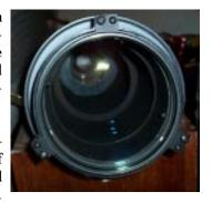
Each pair of screws consists of one "pull" screw which screws into the metal collar and actually holds the front lens cell in the mounting ring. The second screw of each pair is the "push" screw which pushes the lens cell out from the mounting ring allowing you to adjust the "tilt" of the lens cell so that it is perpendicular to the optical axis of the OTA.
