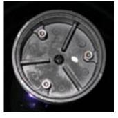
Turn on the laser or use your cross-hair eyepiece to verify that the mark you just made on the secondary is under the cross-hair or the laser dot. If it is not, adjust the secondary by loosening the allen screws holding the cell and moving the entire cell forward or backwards.
