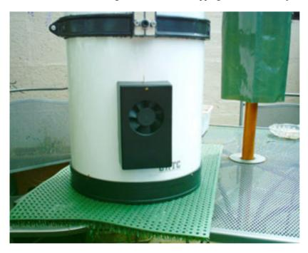
After the holes are cut within the OTA position the plastic fan box over the holes so the path of the airflow will be introduced into the OTA. Mark around the plastic box onto the OTA with a pencil mark – this can come off later.
