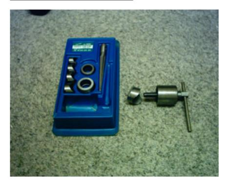
This is the chassis hole punch set - used to make the 3 holes in the OTA. You need to make <u>three</u> overlapping holes, which must be no wider than the base of the plastic box you use to house the fan unit.
